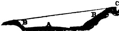
Fig. 149—Cross section of a road in excavation. A, road-surface; B, side slopes. C, top surface-drain.
